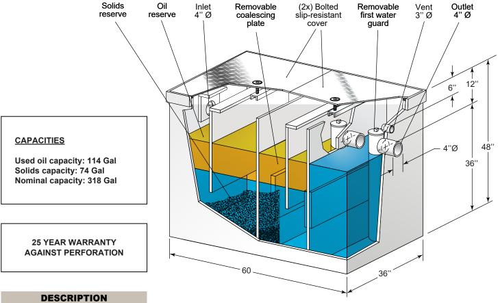
Copolymer polypropylene oil interceptor, capacity of 30 USGPM [114 L/min]. Includes 114 US gal used oil reserve, 75 US gal solids reserve, inlet flow regulator, removable baffles, fixed baffles with removable coalescing plates, water seal equipped with a cleanout, and (2x) 1/4 in. thick slip-resistant aluminum covers with sealing gaskets.
