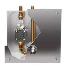
Note: Possibility to install the hydro-pneumatic valve at a maximum distance of 3 m (10 feet) of the push-button actuator (ex: in a suspended ceiling). Minimum dynamic pressure required is 15 psi.
