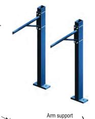
Threaded hole 10-24 with leveling screw
