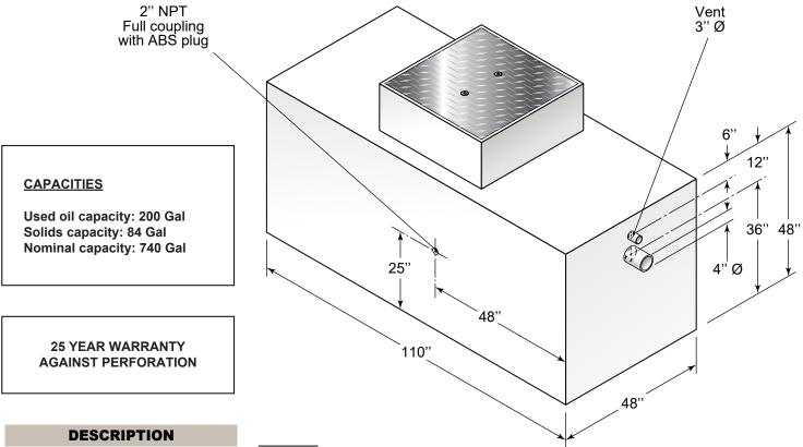
Copolymer polypropylene oil interceptor (3/4" thickness), capacity of 150 USGPM [570 L/min], integrated used oil reserve of 200 US gal, solids reserve of 84 US gal, removable baffle, fixed baffle with removable coalescing plate, water seal equipped with a cleanout, (2x) 3" Ø vents, and (2x) 1/4" thick slip-resistant aluminum covers with sealing gaskets.
